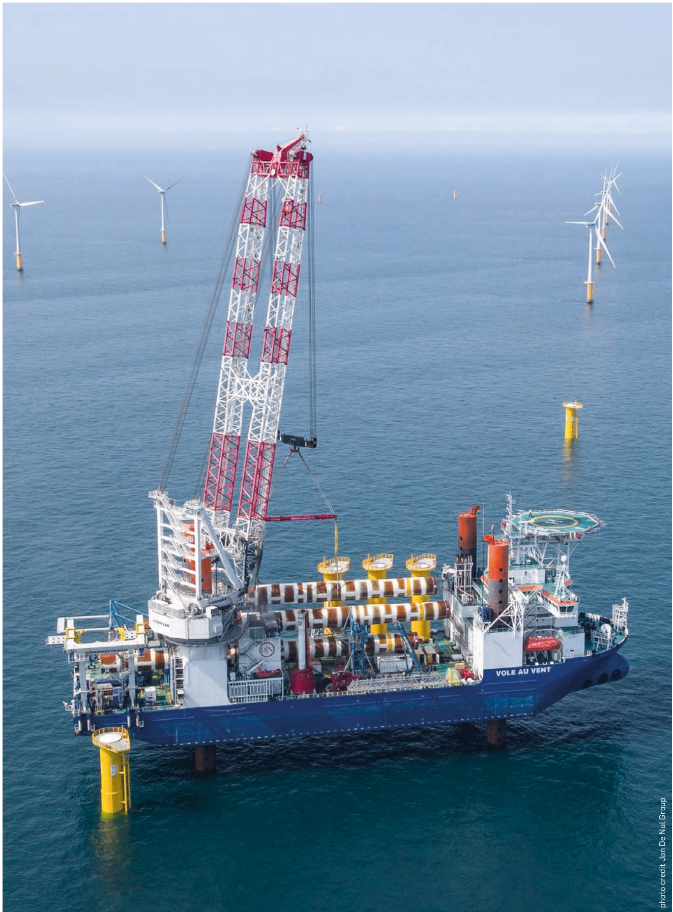
Offshore Jack-up Installation Vessel Vole au Vent 4 x SCD 560 (2600 kW each), 3 x STT 3030 (2500 kW each)
