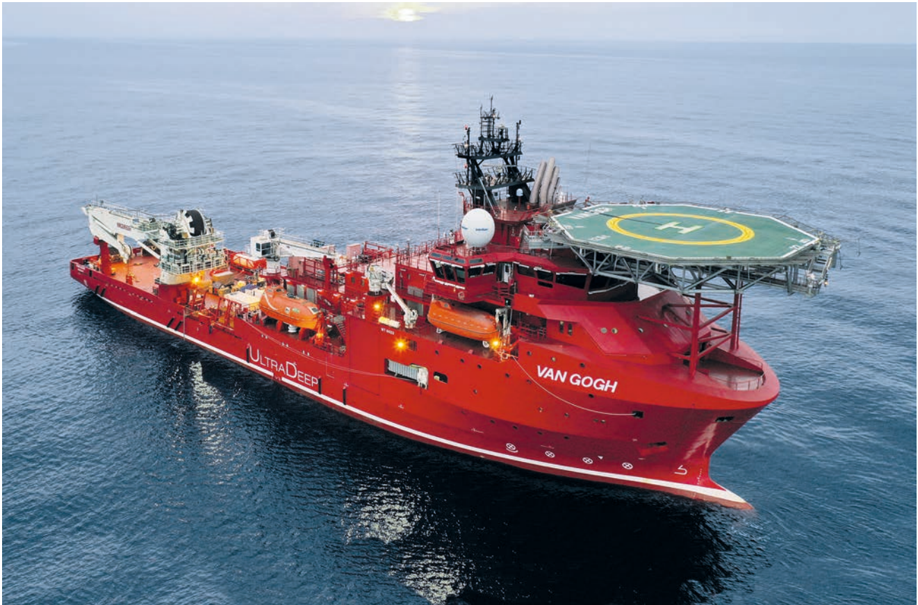
Diving Support Construction Vessel Van Gogh 2 x SRP 630 (3000 kW each), 1 x SRP 340 R (1200 kW), 3 x STT 6 CP (1800 kW each)
