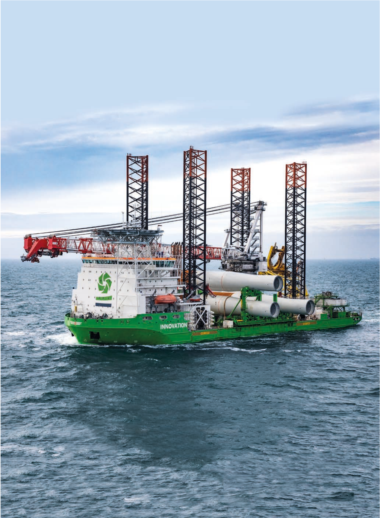
DP2 Offshore Installation Vessel Innovation 4 x SRP 560 (3500 kw each), 3 x STT 3030 (2800 kw each)
