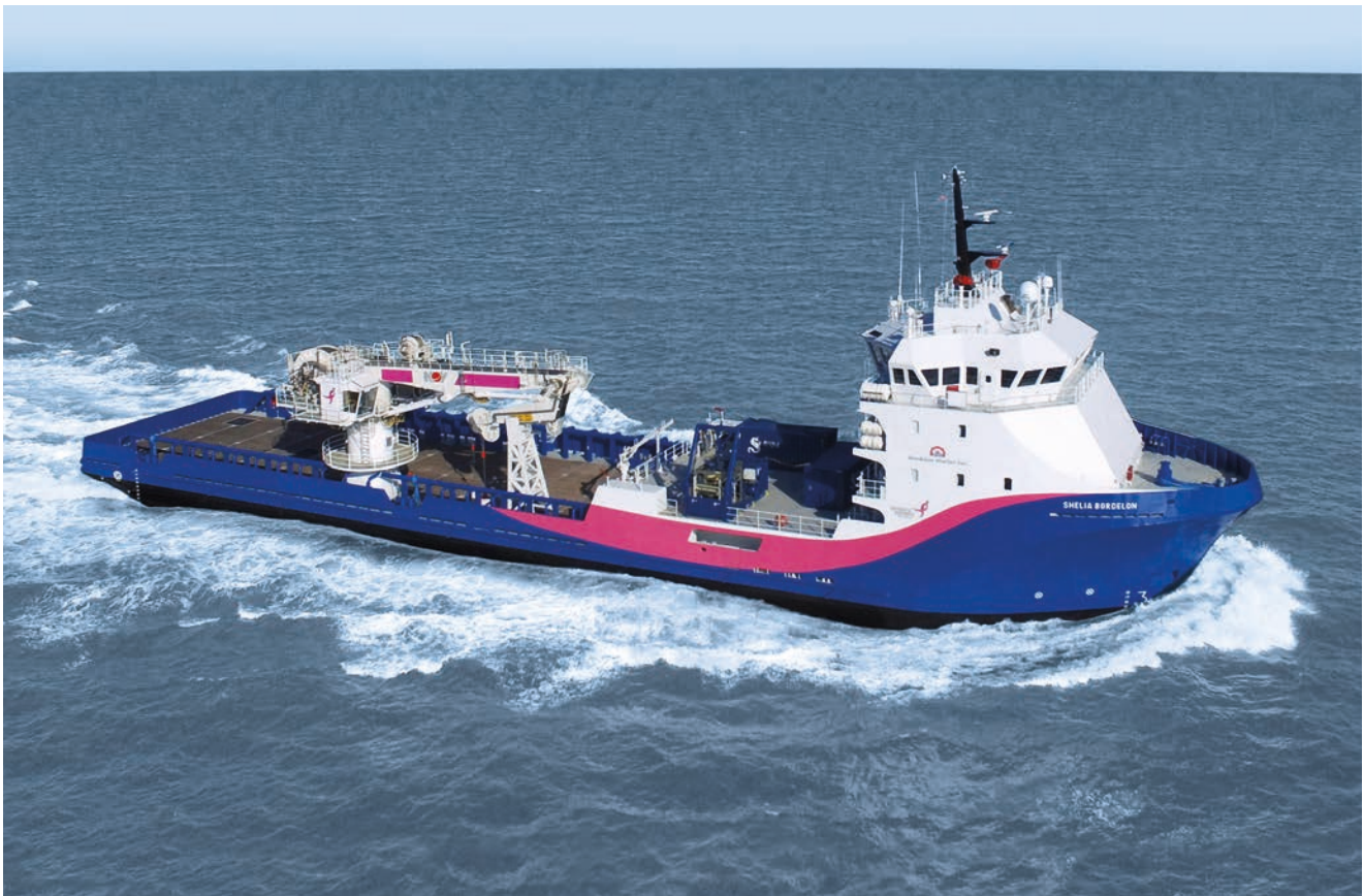
Offshore Support Vessel Shelia Bordelon 2 x SRP 1215 (1641 kW each), 2 x STT 2 (700 kW each)
